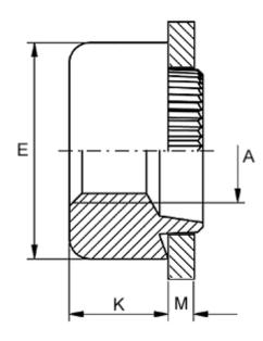
Female thread A = M12Height K = 10.0Outer diameter E = 25.0Plate thickness = 0.5 to 0.6
